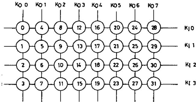
Multi-press of key No. 20 and one of key Nos. 21, 22, 23 may be done, with no priority given in key entry. When the two keys are kept pressed, a series of pulses will be output according to each key entry. If multi-press of keys which are not allowed multi-press is done, no output will be delivered.
