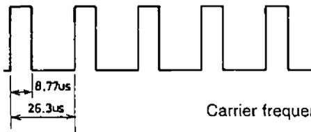
Carrier frequency =  $1/12 f_{OSC} \approx 38 \text{ kHz}$
