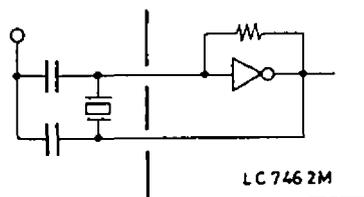
To minimize power dissipation, the oscillator stops oscillating except when key operation is performed.
