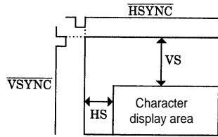
The vertical display start position is set by the 6 bits VP0 to VP5.
