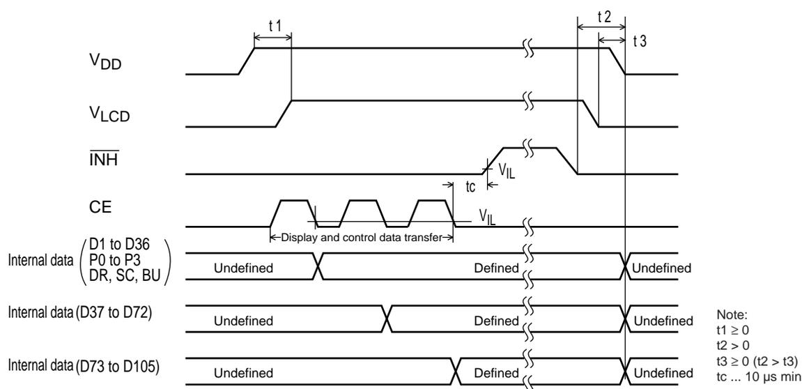
Note: At the LC75833JE, the display data D34 to D36, D67 to D72, D103 to D105 must be set to 0.
