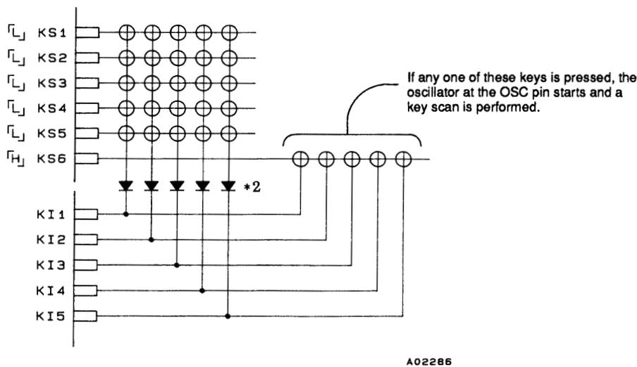
\*2: These diodes are required to reliably recognize events in which three or more of the keys on the KS6 line are pressed at the same time.
