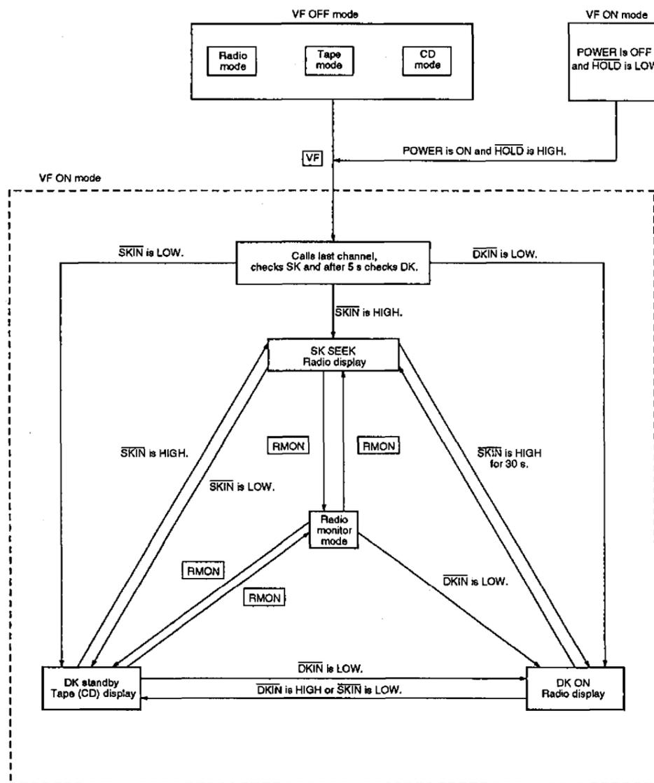
Figure 20. VF mode flowchart
