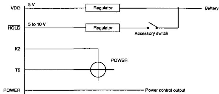
Figure 23. **POWER** key power supply configuration
