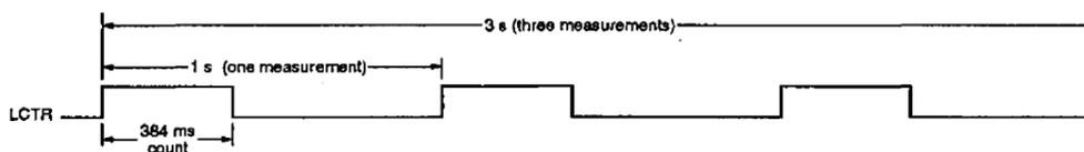
Figure 15. LCTR frequency measurement timing
