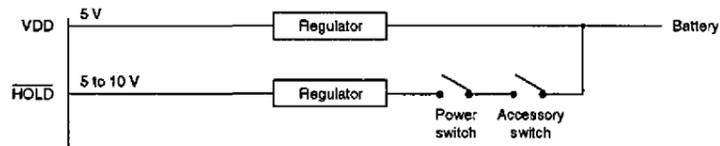
Figure 24. Power supply switch configuration
