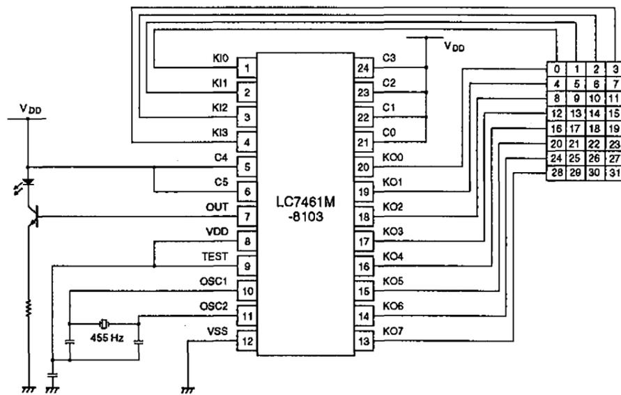
Figure 25. Remote control circuit
