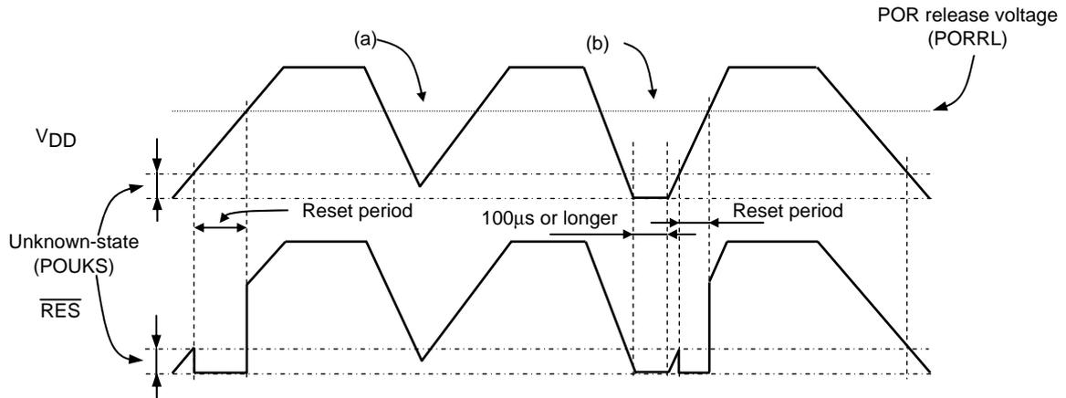
Figure 7 Waveform observed when only POR is used (LVD not used)
