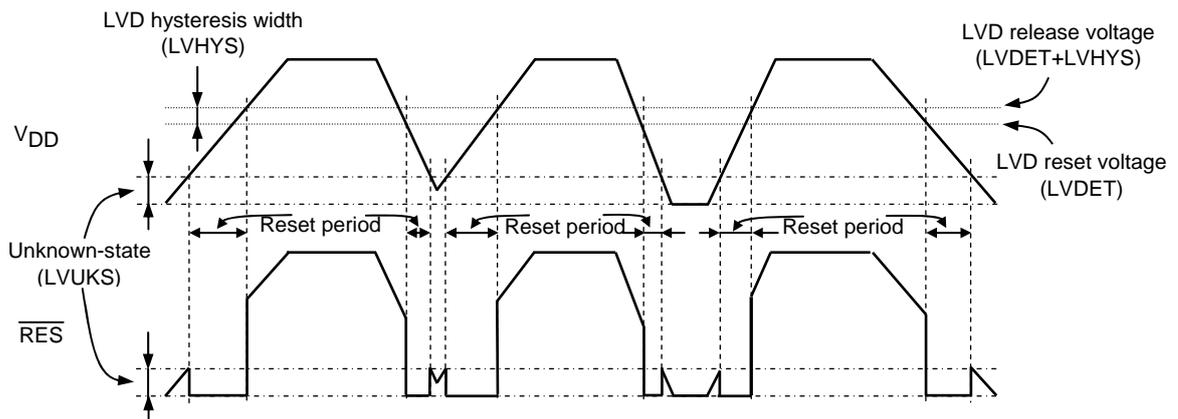
Figure 8 Waveform observed when both POR and LVD functions are used
