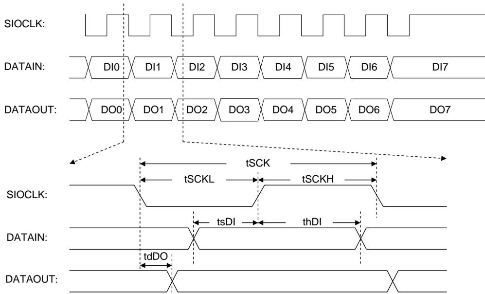
Figure 5 Serial I/O Output Waveforms
