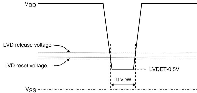
Figure 9 Low voltage detection minimum width
