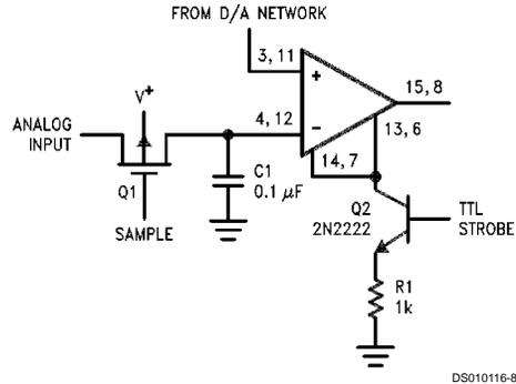
\*Typical input current is 50 pA with inputs strobed off
