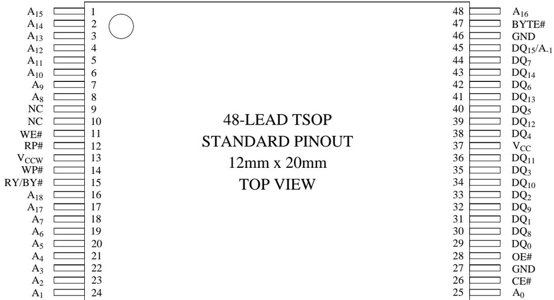
Figure 2. TSOP 48-Lead Pinout
