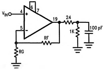
**FIGURE 3. Driving Capacitive Loads**
