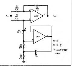
**Differential Input Instrumentation Amplifier**
