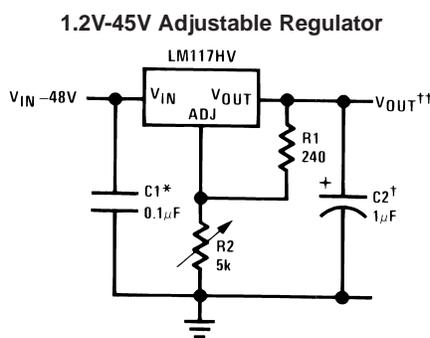
Full output current not available at high input-output voltages
