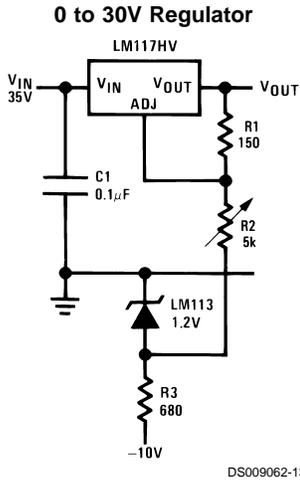
Full output current not available at high input-output voltages
