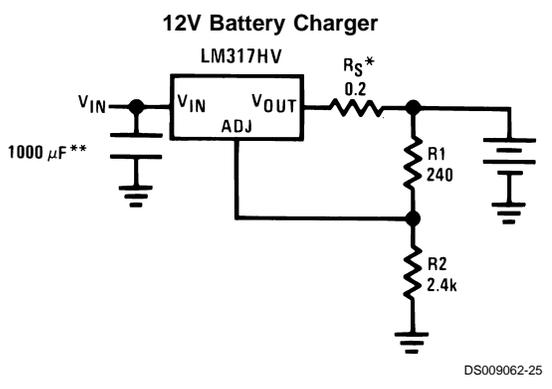
\* $R_S$ —sets output impedance of charger  $Z_{OUT} = R_S \left( 1 + \frac{R_2}{R_1} \right)$
