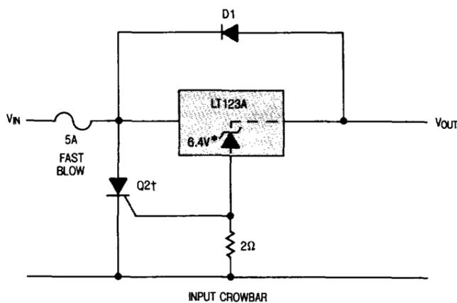
† Q2 AND D1 MUST WITHSTAND LARGE SURGE CURRENTS UNTIL THE 5A FUSE BLOWS. PEAK SURGE CURRENT IS LIMITED ONLY BY THE FUSE, WIRING, AND FILTER CAP RESISTANCE.
