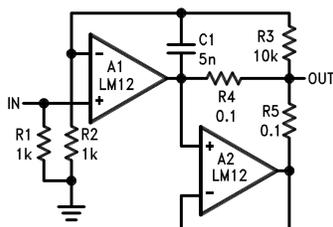
This connection allows increased output capability without requiring a separate control amplifier. The output buffer, A<sub>2</sub>, provides load current through R<sub>5</sub> equal to that supplied by the main amplifier, A<sub>1</sub>, through R<sub>4</sub>. Again, more output buffers can be added.
