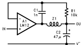
The LM12 can be made stable for all loads with a large capacitor on the output, as shown above. This compensation gives the lowest possible closed-loop output impedance at high frequencies and the best load-transient response. It is appropriate for such applications as voltage regulators.
