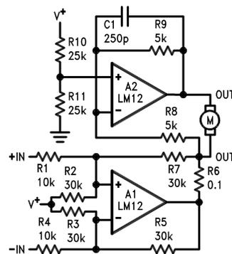
Although op amps are usually operated from dual supplies, single-supply operation is practical. This bridge amplifier supplies bi-directional current drive to a servo motor while operating from a single positive supply. The output is easily converted to voltage drive by shorting  $R_6$  and connecting  $R_7$  to the output of  $A_2$ , rather than  $A_1$ .
