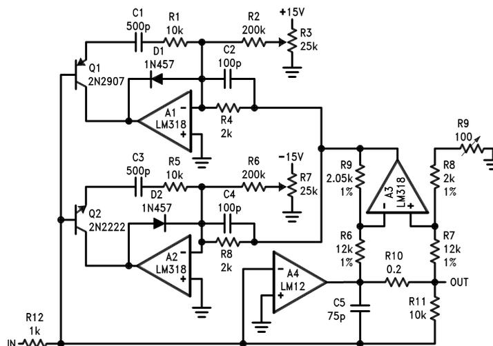
**Note:** Supply voltages for the LM318s are  $\pm 15V$
