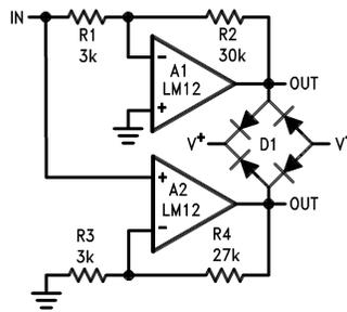
The voltage swing delivered to the load can be doubled by using the bridge connection shown here. Output clamping to the supplies can be provided by using a bridge-rectifier assembly.
