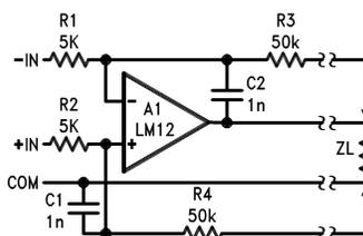
Remote sensing as shown above allows the op amp to correct for dc drops in cables connecting the load. Even so, cable drop will affect transient response. Degradation can be minimized by using twisted, heavy-gauge wires on the output line. Normally, common and one input are connected together at the sending end.
