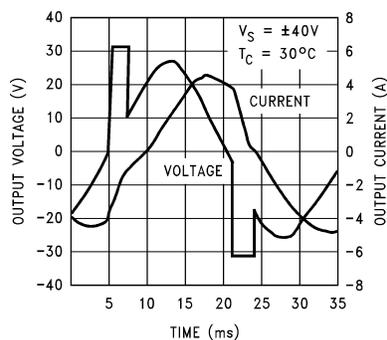
Should the power ratings of the LM12 be exceeded, dynamic safe-area protection is activated. Waveforms with this power limiting are shown for the LM12 driving  $\pm 26V$  at 30 Hz into  $3\Omega$  in series with 24 mH ( $\theta = 45^\circ$ ). With an inductive load, the output clamps to the supplies in power limit, as above. With resistive loads, the output voltage drops in limit. Behavior with more complex RCL loads is between these extremes.
