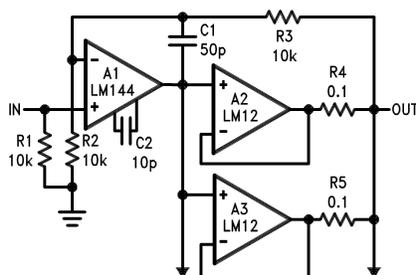
Output drive beyond the capability of one power amplifier can be provided as shown here. The power op amps are wired as followers and connected in parallel with the outputs coupled through equalization resistors. A standard, high-voltage op amp is used to provide voltage gain. Overall feedback compensates for the voltage dropped across the equalization resistors.
