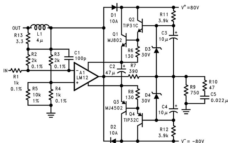
Discrete transistors can be used to increase output drive to  $\pm 70\text{V}$  at  $\pm 10\text{A}$  as shown above. With proper thermal design, the IC will provide safe-area protection for the external transistors. Voltage gain is about thirty.
