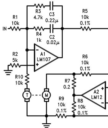
This motor/tachometer servo gives an output speed proportional to input voltage. A low-level op amp is used for frequency shaping while the power op amp provides current drive to the motor. Current drive eliminates loop phase shift due to motor inductance and makes high-performance servos easier to stabilize.
