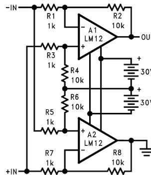
One limitation of the standard bridge connection is that the load cannot be returned to ground. This can be circumvented by operating the bridge with floating supplies, as shown above. For single-ended drive, either input can be grounded.
