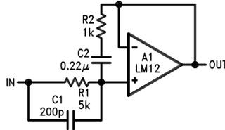
An example of a voltage follower with input compensation is shown here. The  $R_2C_2$  combination across the input works with  $R_1$  to reduce feedback at high frequencies without greatly affecting response below 100 kHz. A lead capacitor,  $C_1$ , improves phase margin at the unity-gain crossover frequency. Proper operation requires that the output impedance of the circuitry driving the follower be well under 1 k $\Omega$  at frequencies up to a few hundred kilohertz.
