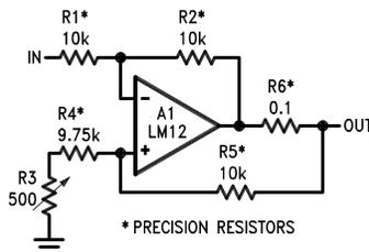
This circuit provides an output current proportional to the input voltage. Current drive is sometimes preferred for servo motors because it aids in stabilizing the servo loop by reducing phase lag caused by motor inductance. In applications requiring high output resistance, such as operational power supplies running in the current mode, matching of the feedback resistors to 0.01% is required. Alternately, an adjustable resistor can be used for trimming.
