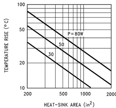
The design of heat sink is beyond the scope of this work. Convection-cooled heat sinks are available commercially, and their manufacturers should be consulted for ratings. The preceding figure is a rough guide for temperature rise as a function of fin area (both sides) available for convection cooling.
