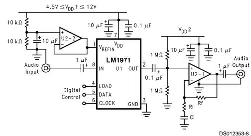
FIGURE 7. Active Reference with Active Gain Buffering
