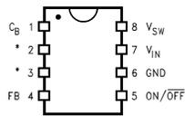
Figure 2. SO-8/DIP Package 8-Lead Package Top View
