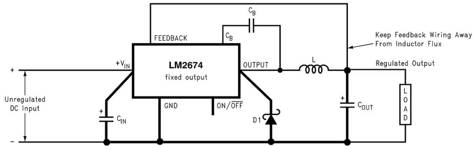
Heavy Lines Must Be Kept Short And Use Ground Plane Construction For Best Results
