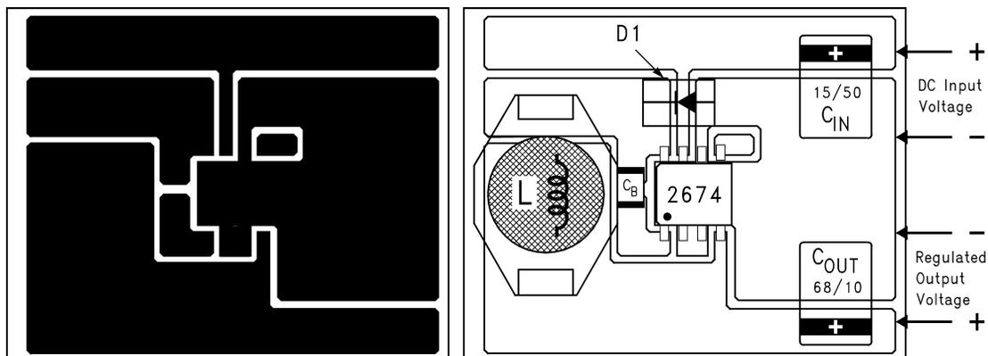
$C_{IN}$  - 15  $\mu\text{F}$ , 25V, Solid Tantalum Sprague, "594D series"
