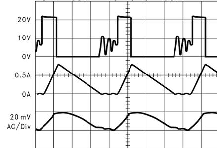
A:  $V_{SW}$  Pin Voltage, 10 V/div.
