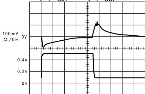
A: Output Voltage, 100 mV/div, AC-Coupled.
