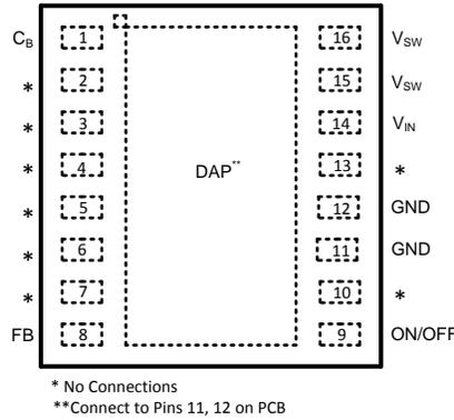
Figure 1. 16-Lead LLP Surface Mount Package Top View
