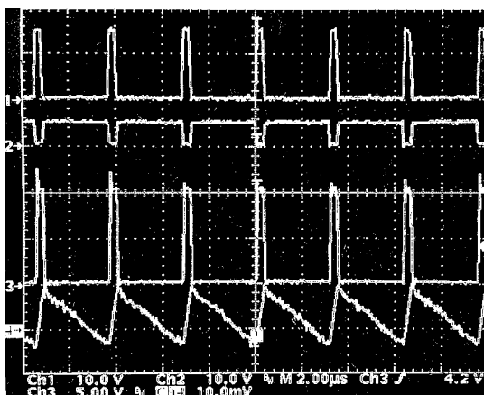
Figure 4. Normal FPWM Mode Operation at Light Loads
