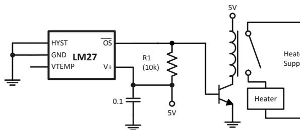
Figure 8. Simple Thermostat
