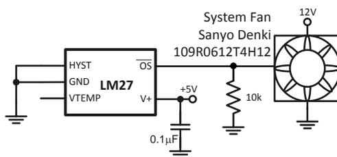
Note: The fan's control pin has internal pull-up. The 10k pull-down sets a slow fan speed. When the output of the LM27A goes low, the fan will speed up.
