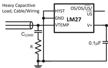
Figure 2. a) R in series with capacitor
