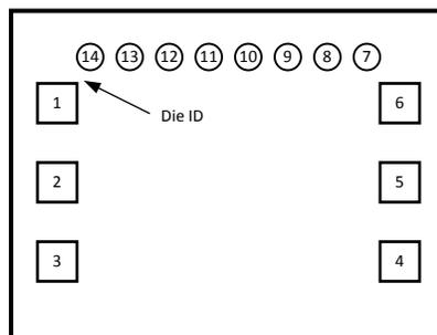
Figure 1. LM27A Bond Pad Layout (TOP VIEW)
