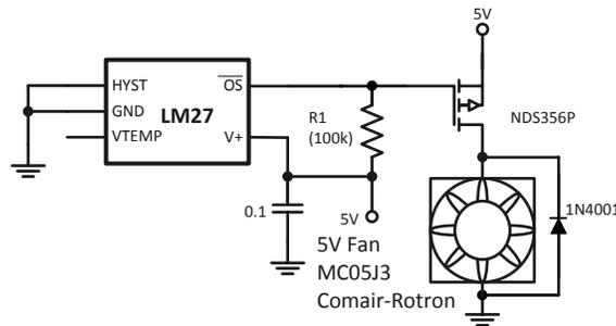
Figure 5. Fan High Side Drive
