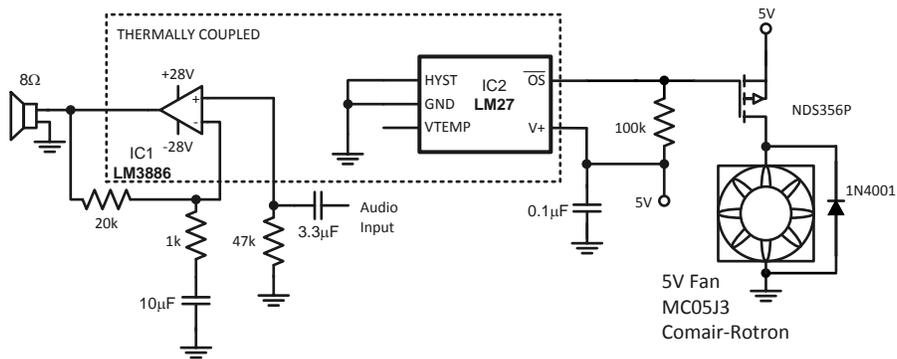
Figure 7. Audio Power Amplifier Thermal Protection
