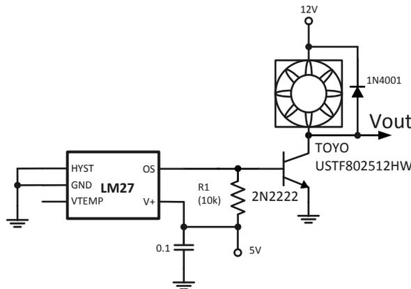
Figure 6. Fan Low Side Drive
