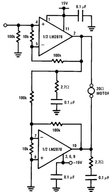
FIGURE 4. LM2878 Servo Amplifier in Bridge Configuration TL/H/7934-8
