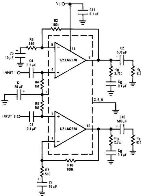
FIGURE 3. Stereo Amplifier with  $A_V = 200$  TL/H/7934-7
