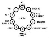
Note: Pin 5 connected to case.
