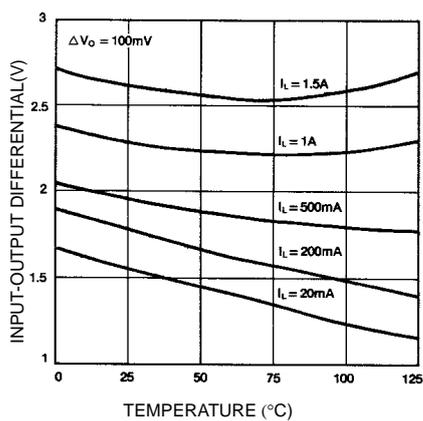
Figure 3. Dropout Voltage
