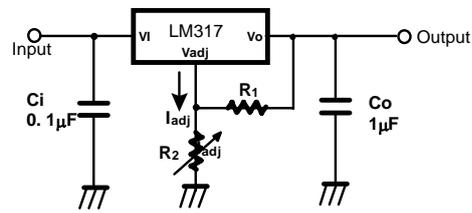
$$V_O = 1.25V (1 + R_2 / R_1) + I_{adj} R_2$$
