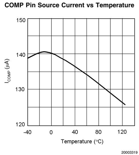
**Typical Performance Characteristics** Unless otherwise specified,  $V_{IN} = 12V$ ,  $T_J = 25^\circ C$ . (Continued)
