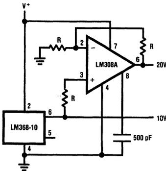
R = Thin Film Resistor Network
