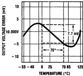
Typical Temperature Coefficient Calculations:
