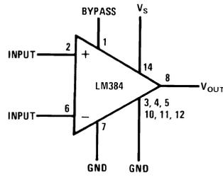
Figure 2. Block Diagram
