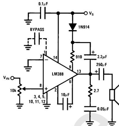
**FIGURE 4. Amplifier with Gain = 200 and Minimum  $C_B$**
