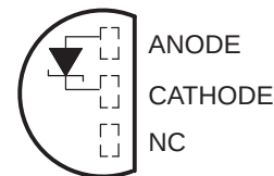
LP (TO-92/TO-226) PACKAGE (TOP VIEW)
