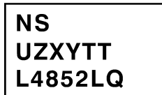
Figure 5. 24 Lead LLP Marking NS: Standard NS Logo U: Wafer Fab Code Z: Assembly Plant Code XY: Date Code TT: Die Traceability L4852LQ: LM4852LQ
