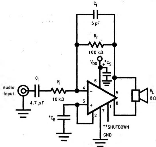
FIGURE 2. Audio Amplifier with  $A_{VD} = 20$
