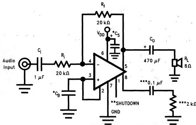
FIGURE 3. Single-Ended Amplifier with  $A_V = -1$
