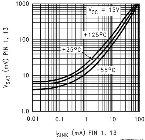
**Discharge Transistor (Pin 1, 13) Voltage vs. Sink Current**
