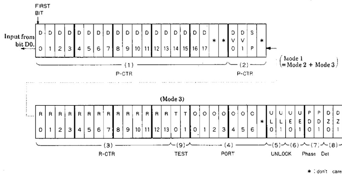
The serial data for controlling the LM7005 consists of 56 bits. After the power on, all the 56 bits must be input to the LM7005 for initialization.
