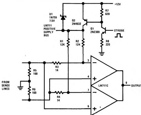
\*Standby dissipation is about 40 mW
