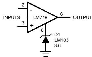
**Figure 4. Voltage Comparable for Driving RTL Logic or High Current Driver**
