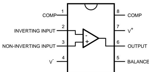
Figure 1. Dual-In-Line Package - Top View
