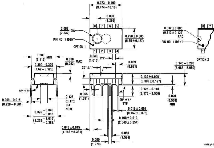
**8-Pin Molded Dual-In-Line Package (N)**
