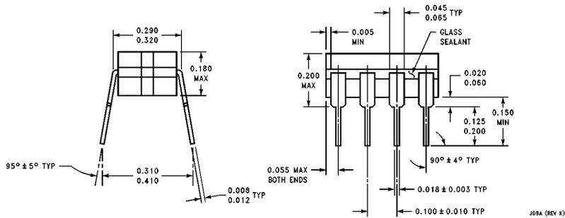
**8-Lead Ceramic Dual-In-Line Package (J)**
