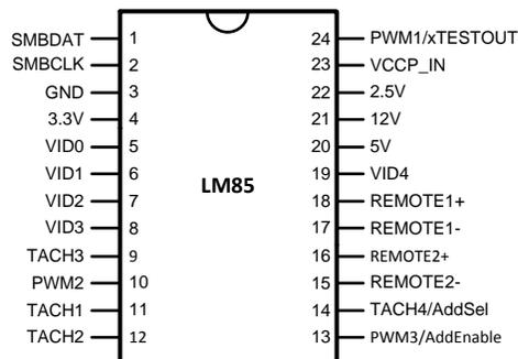
**Figure 1. 24-Pin SSOP - Top View**
