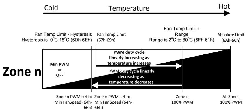
**Figure 2. Fan Activity above Fan Temp Limit****Example for PWM1 assigned to Zone 1:**
