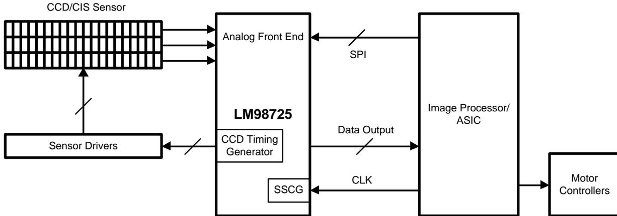
LM98725 Overall Chip Block Diagram
