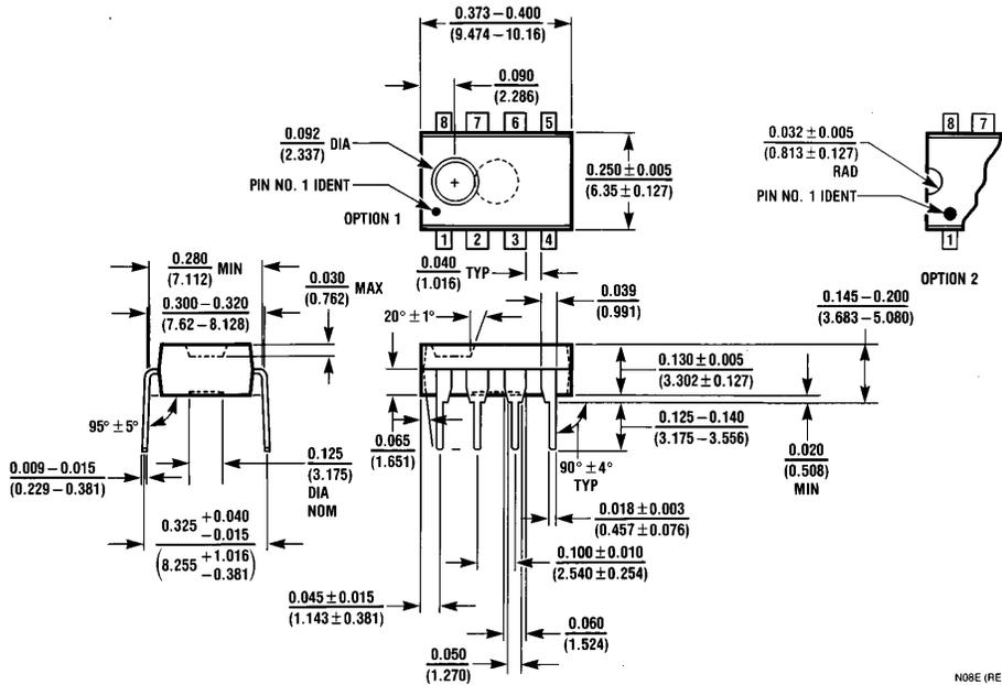
**8-Pin Molded Dual-In-Line Package**
