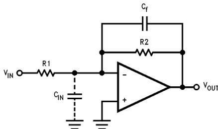
FIGURE 1. Cancelling the Effect of Input Capacitance
