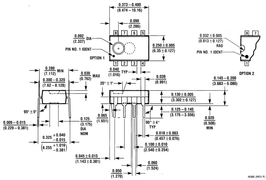
**8-Pin Molded Dual-In-Line Package**
