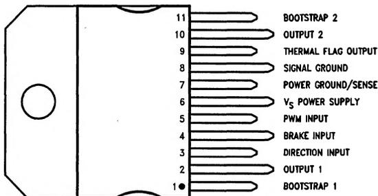
MOUNTING TAB CONNECTED TO GROUND (PIN 7)
