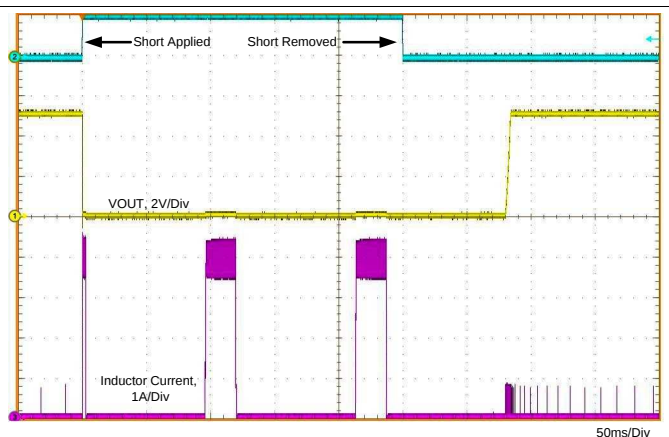
Figure 12. Short-Circuit Transient and Recovery
