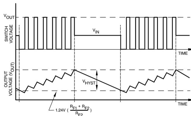
Figure 5. Typical Step-Up Regulator Waveforms
