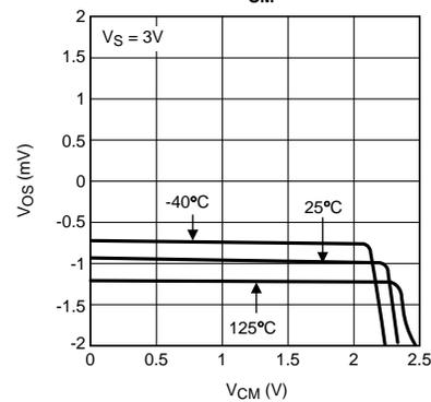
$V_{OS}$  vs.  $V_{CM}$
