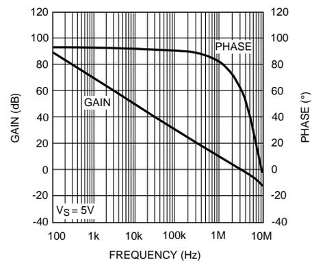
**Figure 1. Open Loop Gain and Phase vs. Frequency**
