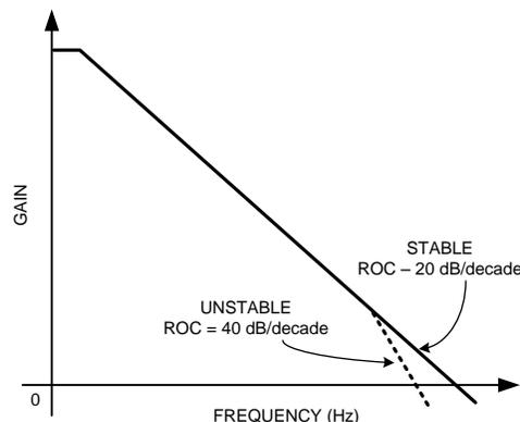
**Figure 5. Gain vs. Frequency for an Op Amp**
