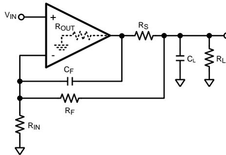
Figure 6. In the Loop Compensation
