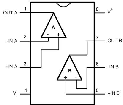
**Figure 3. 8-Pin MSOP (Top View)**
