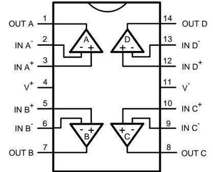
**Figure 4. 14-Pin TSSOP (Top View)**
