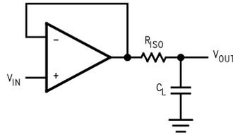
Figure 7. Compensation by Isolation Resistor
