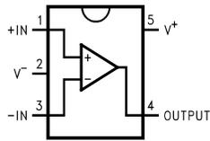
**Figure 2. 5-Pin SC70/ SOT-23 (Top View)**
