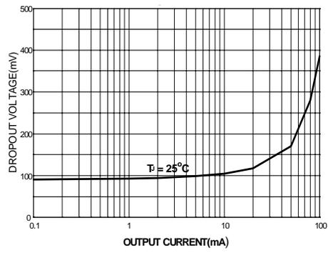
Figure 8. Dropout Voltage
