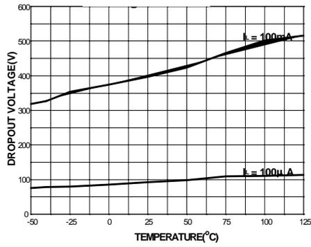
Figure 7. Dropout Voltage
