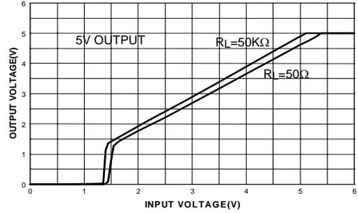
Figure 2. Dropout Characteristics
