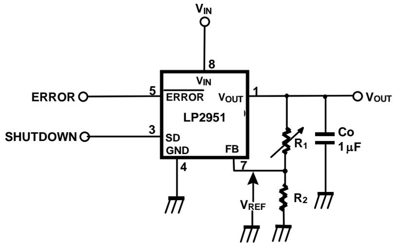
$$V_O = V_{REF} (1 + R_1 / R_2) + I_{FB} R_1$$
