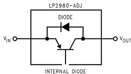
If the output is forced above the input by more than a  $V_{\text{BE}}$ , this diode will become forward biased and current will flow into the output pin and out the input pin. This current must be limited to  $< 100\ \text{mA}$  to prevent damage to the part.
