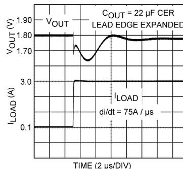
**Figure 21. 22 µF Ceramic Output Capacitor**
