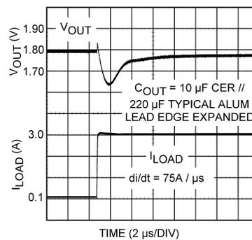
**Figure 23. 10 µF Ceramic Paralleled By 220 µF Generic Aluminum Electrolytic**
