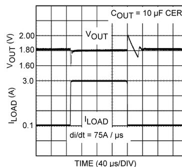
Figure 19. Load Transient Response: 10 μF Ceramic, 75A/μs di/dt
