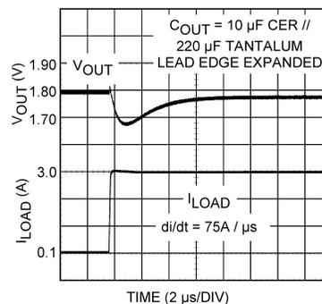
**Figure 24. 10 µF Ceramic Paralleled By 220 µF Tantalum**
