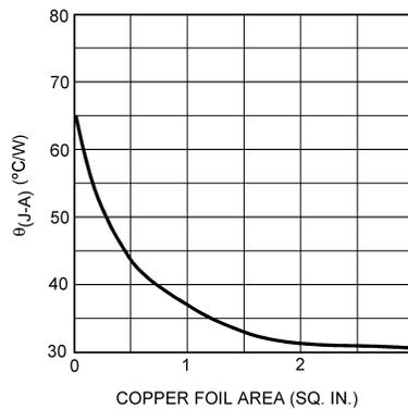
**Figure 26.  $\theta_{JA}$  vs Copper Area for TO-263 Package**
