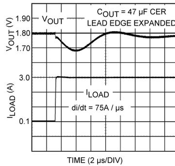
**Figure 22. 47 µF Ceramic Output Capacitor**
