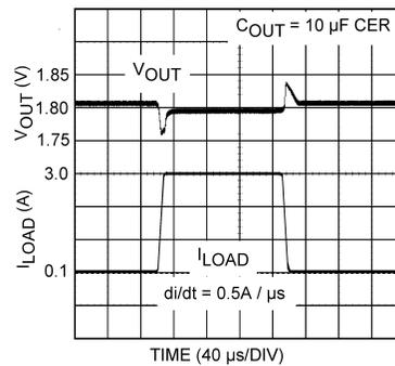
Figure 18. Load Transient Response: 10 μF Ceramic, 0.5A/μs di/dt
