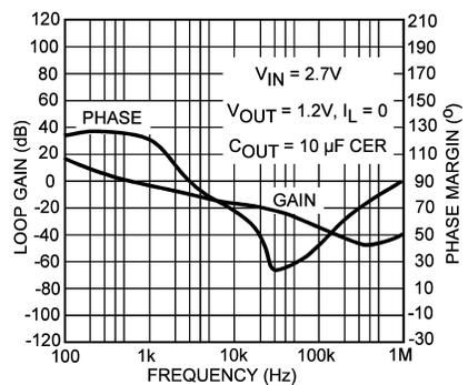
Figure 17. Gain-Bandwidth Plot for No Load
