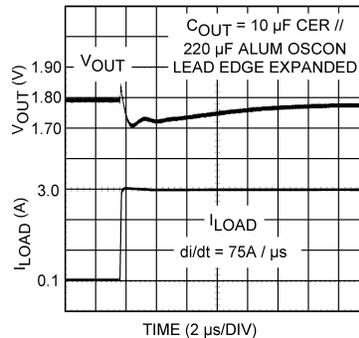
**Figure 25. 10  $\mu\text{F}$  Ceramic Paralleled By 220  $\mu\text{F}$  OSCON**
