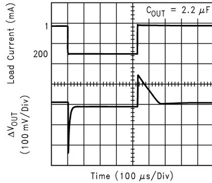
**Typical Performance Characteristics** Unless otherwise specified,  $C_{IN} = 1 \mu\text{F}$  ceramic,  $C_{BYP} = 0.01 \mu\text{F}$ ,  $V_{DD} = V_{OUT} + 0.2\text{V}$ ,  $T_A = 25^\circ\text{C}$ , Enable pin is tied to  $V_{DD}$ . (Continued)
