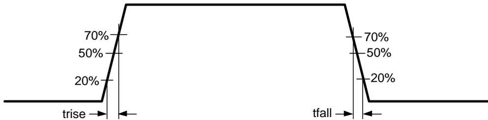
Figure 4. Output Transition Time (A and B Side)
