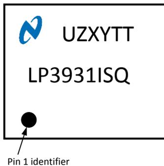
Figure 3. Package Mark—Top View
