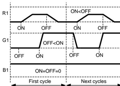
Figure 20. Example Blinking Waveforms
