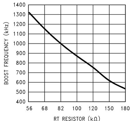
Figure 11. Boost Frequency vs RT Resistor
