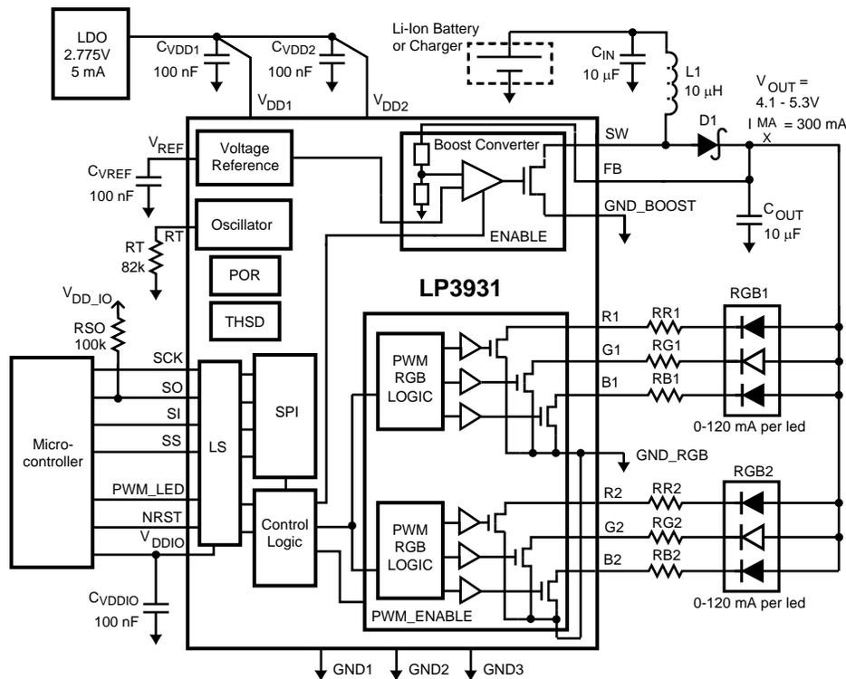
Figure 4. LP3931 Block Diagram
