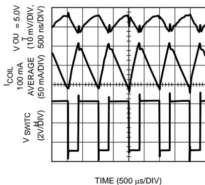
Figure 14. Boost Typical Waveforms at 100 mA Load
