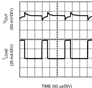
**Figure 17. Boost Load Regulation, 50 mA-100 mA**
