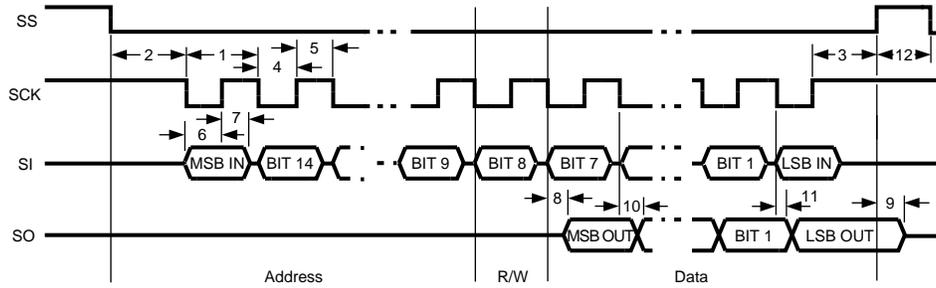
Figure 7. SPI Timing Diagram
