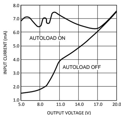
Figure 21. Autoload Effect on Input Current, No Load
