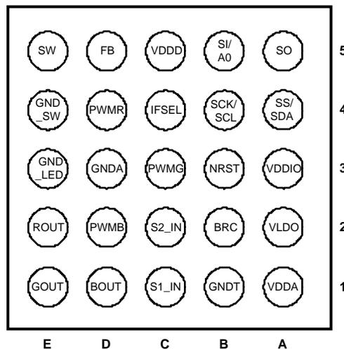
**Figure 2. DSBGA-25 Package, Large Bump Bottom View
