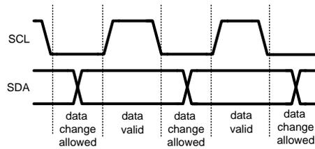
**Figure 26. I<sup>2</sup>C Signals: Data Validity**
