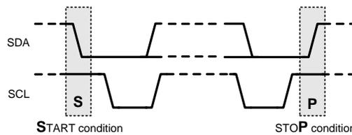
**Figure 27. I<sup>2</sup>C Start and Stop Conditions**
