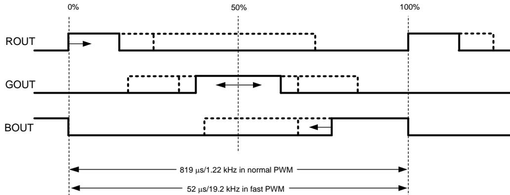
Figure 13. Pulse positions in the PWM cycle
