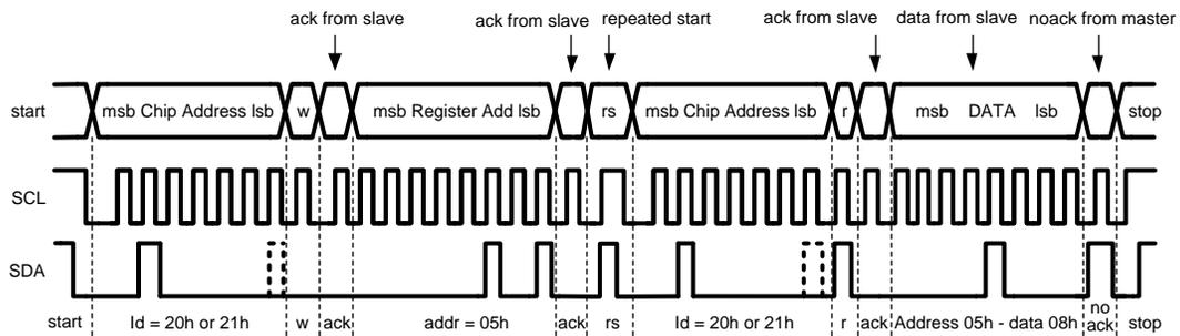
Figure 30. I<sup>2</sup>C Read Cycle
