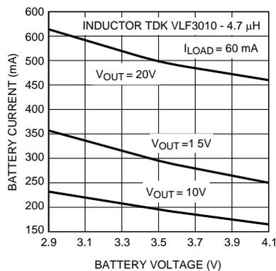
Figure 20. Battery Current vs. Voltage
