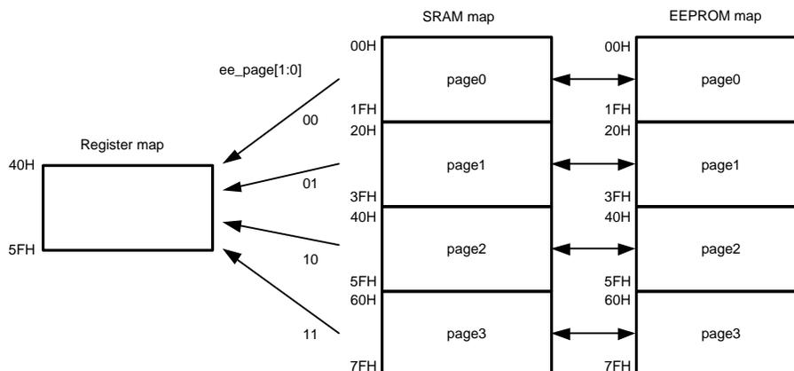
EEPROM content is copied into SRAM always when the chip is taken from stand-by mode to active mode. Copying to SRAM can also be made during operation by writing the **<ee\_read>** bit high and low in the **EEPROM control** (0DH) register. For reading the data from the SRAM, the page number must be set with **<ee\_page[1:0]>** bits and the page read from addresses 40H – 5FH.
