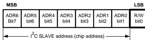
**Figure 28. I<sup>2</sup>C Chip Address**
