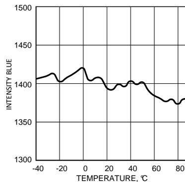
Figure 11. Compensated Blue LED Intensity vs. Temperature
