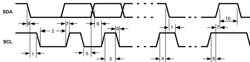
Figure 31. I<sup>2</sup>C Timing Diagram
