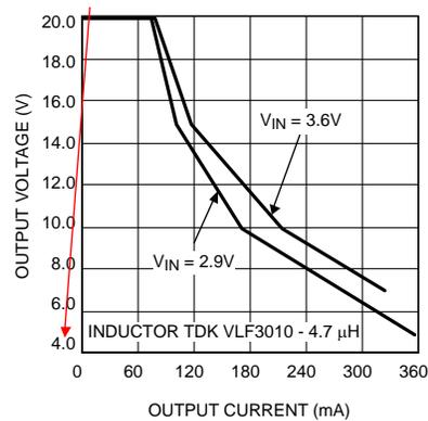
Figure 19. Boost Max. Output Voltage vs. Current
