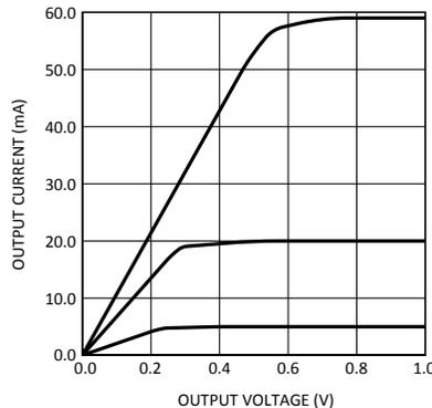
Figure 15. V<sub>SAT</sub> vs I<sub>LED</sub>
