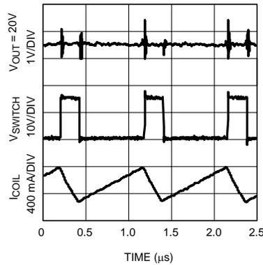
Figure 18. Boost Typical Waveforms at 60 mA Load
