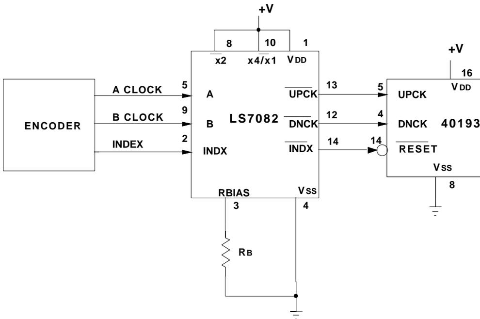
FIGURE 6. A TYPICAL APPLICATION IN x4 MODE
