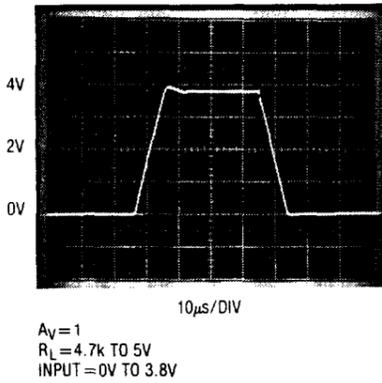
**Large Signal Transient Response,  $V_S = 5\text{V}, 0\text{V}$**
