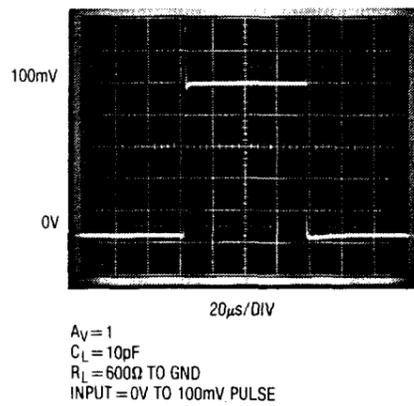
**Small Signal Transient Response,  $V_{CC} = \pm 2.5\text{V to } \pm 15\text{V}$**
