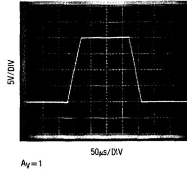
**Small Signal Transient Response,  $V_S = 5\text{V}, 0\text{V}$**
