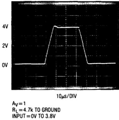
**Large Signal Transient Response,  $V_S = \pm 15\text{V}$**
