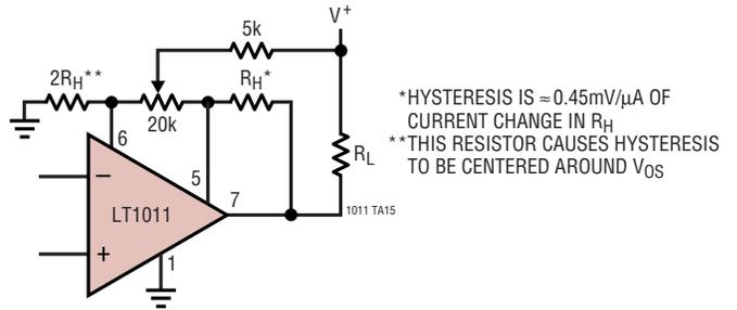
**Direct Strobe Drive When CMOS\* Logic Uses Same V+ Supply as LT1011**
