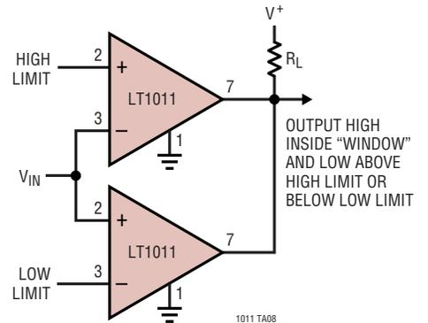
OUTPUT HIGH INSIDE "WINDOW" AND LOW ABOVE HIGH LIMIT OR BELOW LOW LIMIT
