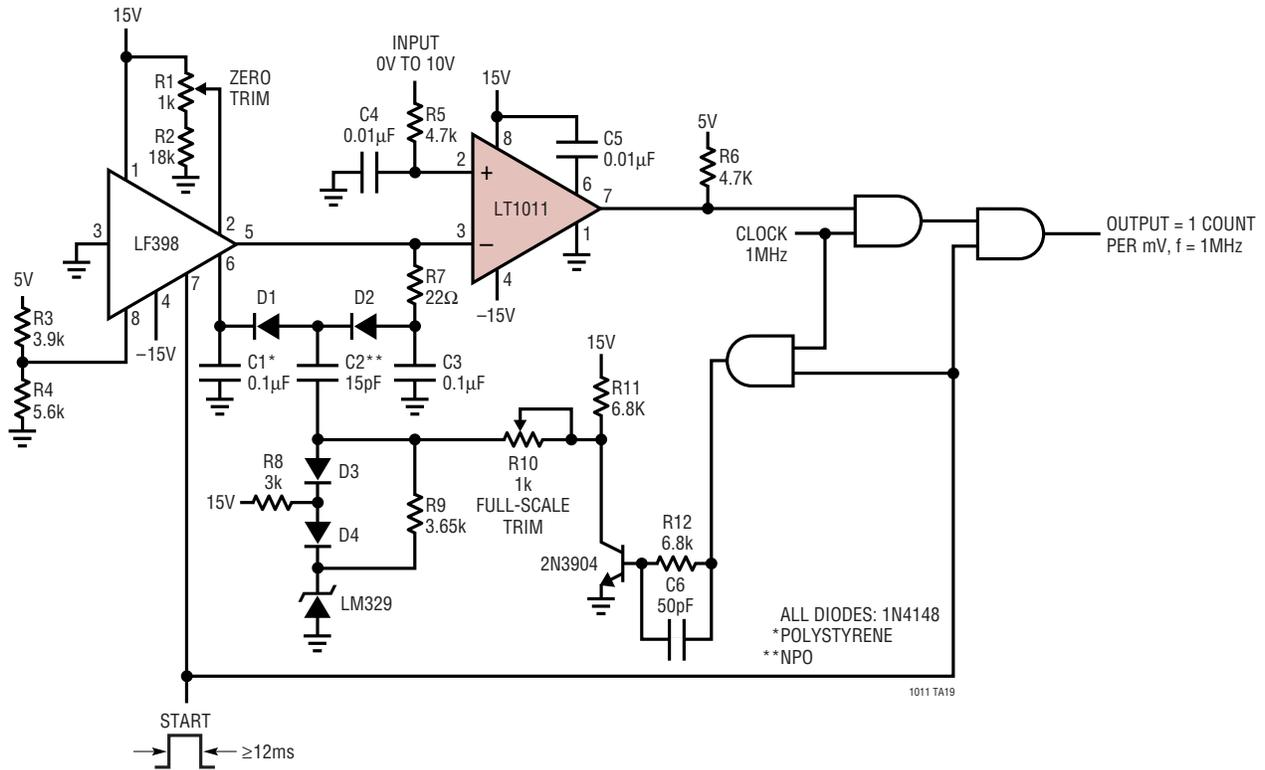
Capacitance to Pulse Width Converter
