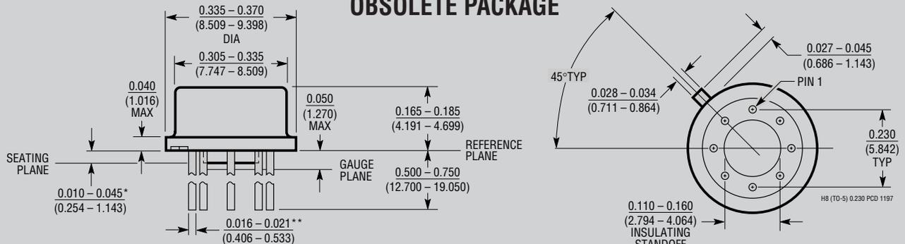
\* LEAD DIAMETER IS UNCONTROLLED BETWEEN THE REFERENCE PLANE AND 0.045" BELOW THE REFERENCE PLANE
